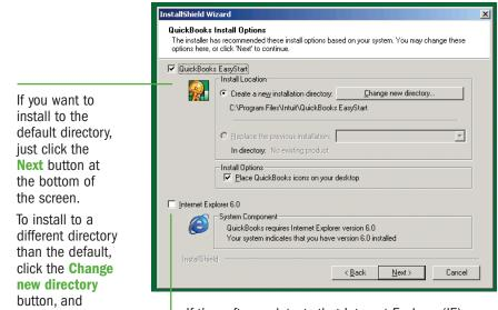
If the software detects that Internet Explorer (IE) version 6.0 is not installed on your computer, this checkbox is selected. Do not clear this checkbox if it is selected. IE 6.0 is needed for EasyStart to run properly.
